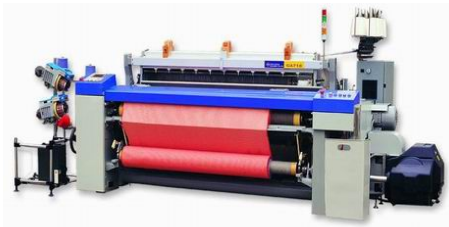
Fig 2.2 Modern air-jet weaving machine
