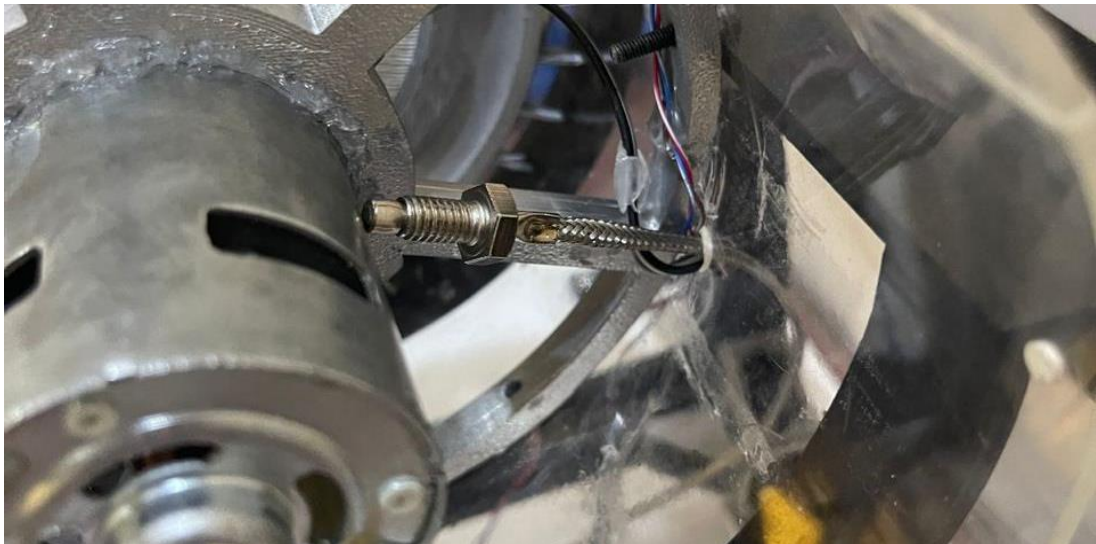
Figure 6.3 Actual K-type and Chamber Temp. Sensor Placement
