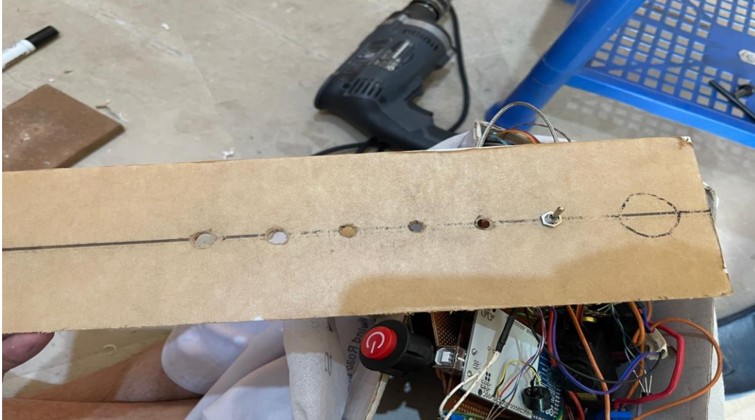
Figure 4.7 Drilling for Toggle Switches
