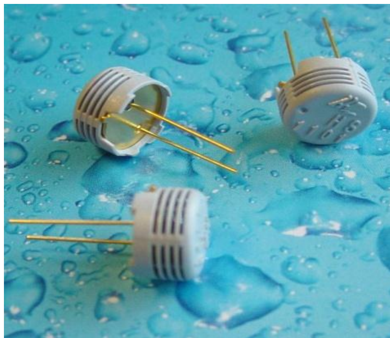
Figure5: Temperature and Humidity Sensors
