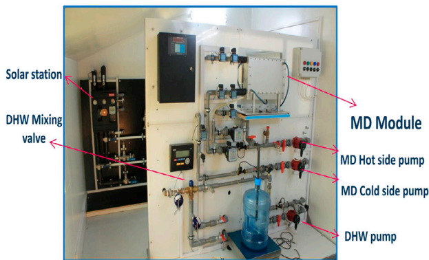
Fig. 6. MD system with solar station.
